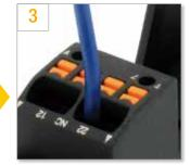
Release the flat-blade screwdriver. Connection is completed. Pull lightly to make sure it is firmly in place.
