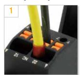
Push the pusher using a flat blade screwdriver.
