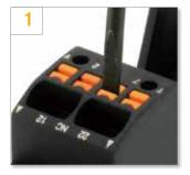
Hold down the pusher with a flatblade screwdriver.
