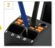
While holding down the pusher, insert the wire to the back of the wire port.
