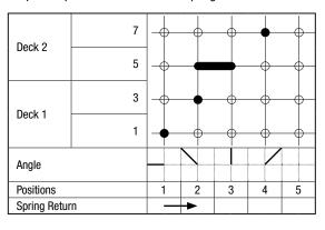
2. Specify contact operation at each operator position Indicate the required operation of all contacts at each operator position using the following symbols.
