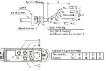
(1)Connect wires starting from the lower terminals
