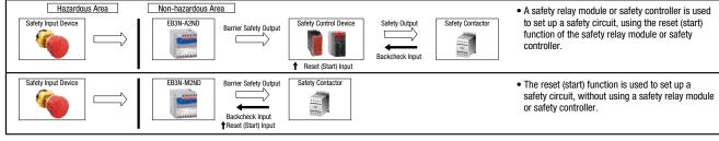
Connection with multiple safety input devices, capable of monitoring up to 5 contact operations, compliant with Category 3 For monitoring operating statuses of safety input devices located in a non-hazardous area
