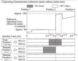
Note: The operating force of the enabling switch with rubber boot depends on the ambient temperature.
